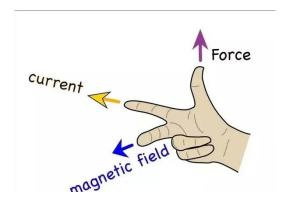
The direction of the magnetic force can be found by using the right hand rule.
