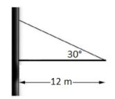
The rod doesn't move, it means that it is in the state of equilibrium and sum of all forces in X and Y directions is equal to zero, or:
