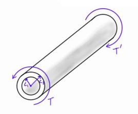
We have hollow shaft with outer radius  $c_2 = 140$  mm and inner radius  $c_1 = 125$  mm. Also we know the allowable shearing stress is  $\tau_{al} = 100$  MPa. To find the maximum torque we can use equation for shear stress:
