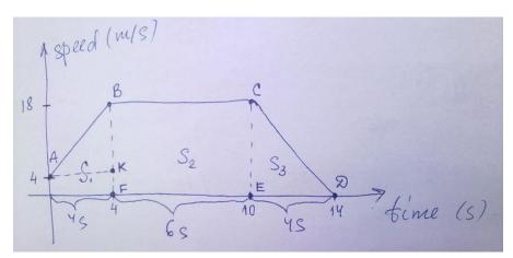
b. The acceleration of the car during the first 4s equal to the slope of the line AB:
