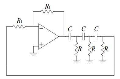
Figure above shows the circuit for a phase shift oscillator, in which the feedback circuit employs three cascaded RC sections to shift the phase by 180°. An additional shift of 180° is obtained by using an inverting amplifier.
