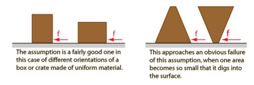
While exceptions exist, the assumption has enough validity to be useful in many circumstances. For example, it implies that wide tires will not in general give better traction than narrow tires, and will not change the normal braking distance for a car. Better traction can be obtained with wide tires, or tires with lower pressure, if the pressure changes the coefficient of friction, as on a surface of snow.
