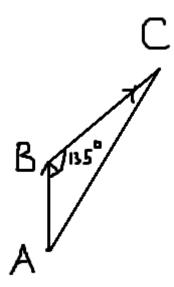
where AB = 3, BC = 5,  $\angle ABC = 135^{\circ}$ . The resultant displacement is AC.
