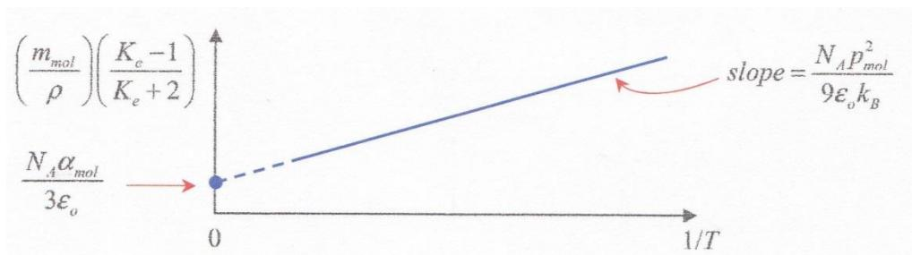
Dielectric constant and electric susceptibility of a polar dielectric are inversely proportional to the absolute temperature  $T$ . Non-polar dielectrics have no such temperature dependence.
