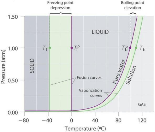
Freezing is the process of transformation liquid phase into solid and evaporation (boiling) - liquid phase into vapour. That's why easier to measure freezing temperature not boiling.
