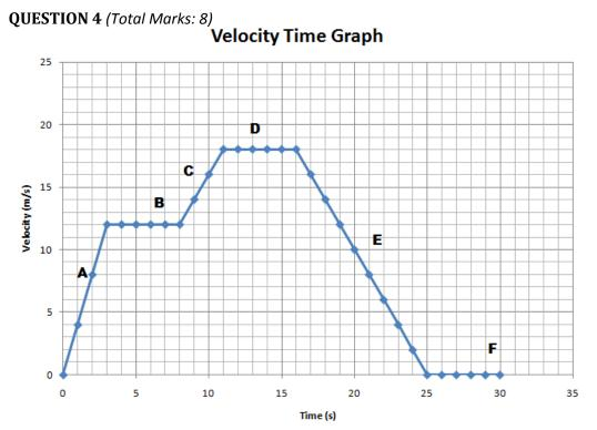
The *Velocity vs Time* behavior for an object in motion is shown in the graph above. (a) Identify the region or regions (A, B, C, D, E, F) in which the object is accelerating. **Answer.** The object accelerates on the regions A and C.
